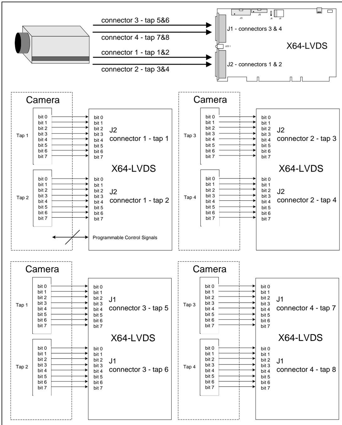
**If the camera has eight channels or taps that output 8-bits per pixel:**
