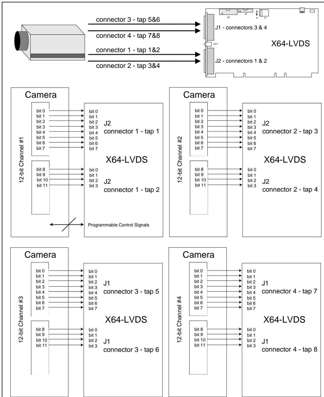
**If the camera has four channels that output 12-bits per pixel:**
