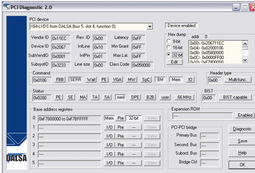
Clicking on the **Diagnostic** button opens a new window with the diagnostic report. From the PCI Bus Number drop menu select the bus number that the X64-LVDS is installed in. In this example the computer PCI expansion slots are identified as bus 5.
