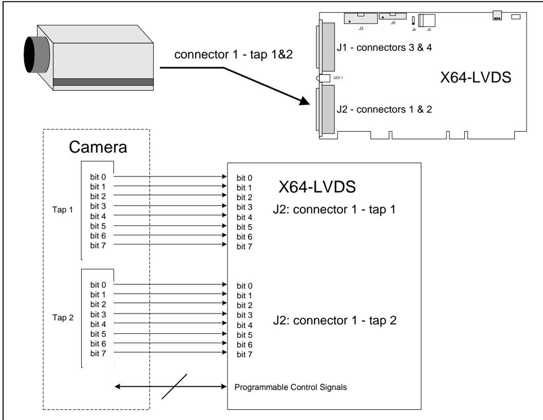
**If the camera has two channels or taps that output 8-bits per pixel:**
