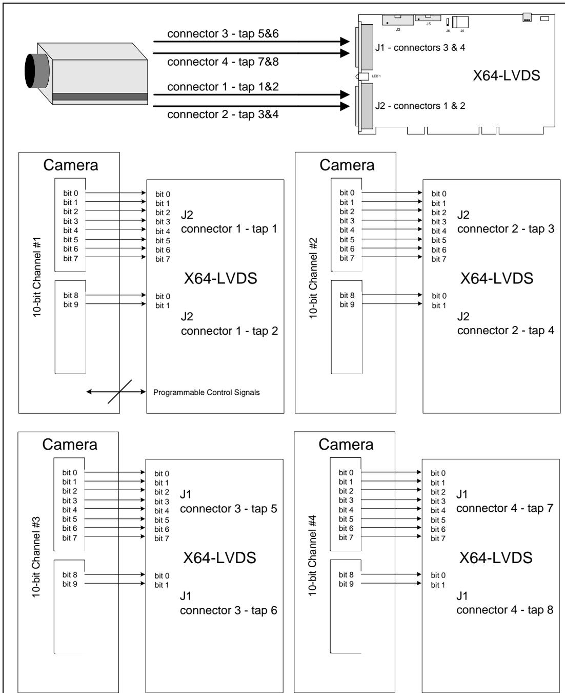
**If the camera has four channels that output 10-bits per pixel:**
