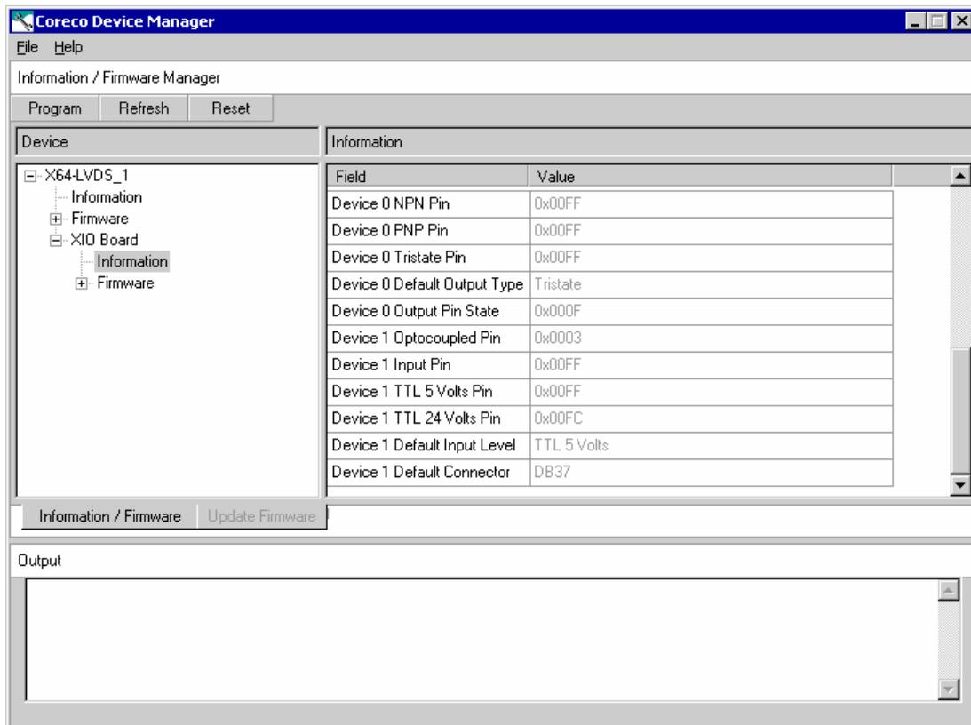
The XIO information screen shows the current status of **Device 0**—the output device, and **Device 1**—the input device. A few items are user configurable for X-I/O board power up state. Click on the item to display a drop list of available capabilities, as described below.
