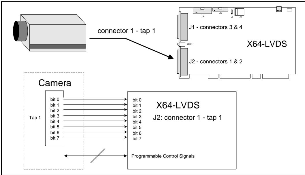
**If the camera has one channel or tap that outputs 8-bits per pixel:**
