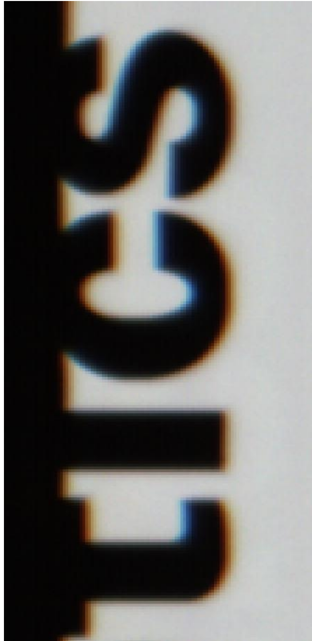
30° Camera Angle, 8k Camera, 80mm lens, 20um Object Pixel, Spatial Correction =9.2, No Parallax Correction
