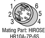
Figure 8: Hirose 6-pin Circular Male—Power Connector and Table 6: Hirose Pin Description
